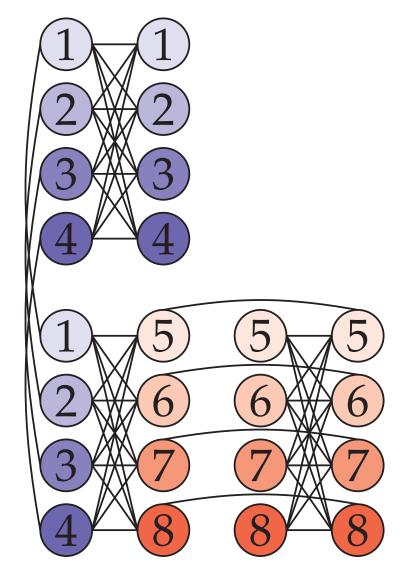
Qubits are sparsely connected in the D-Wave hardware (left side above shows connection pattern). Connected problem variables must be mapped to groups of qubits that share at least one hardware connection. The right side above shows how to map eight mutually connected problem variables to qubits: qubits with the same number (and color) represent the same problem variable. All qubits representing the same variable must be connected in a chain.
