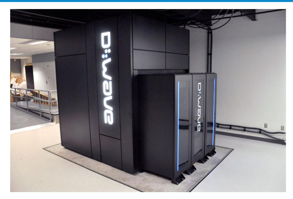
The adiabatic quantum annealer by the Canadian company D-Wave exploits a limited form of quantum computing to solve NP-hard optimization problems. Its Niobium circuits are placed in a vacuum and cooled down to a temperature close to absolute zero. Under those conditions, Niobium becomes superconducting and quantum effects appear.
